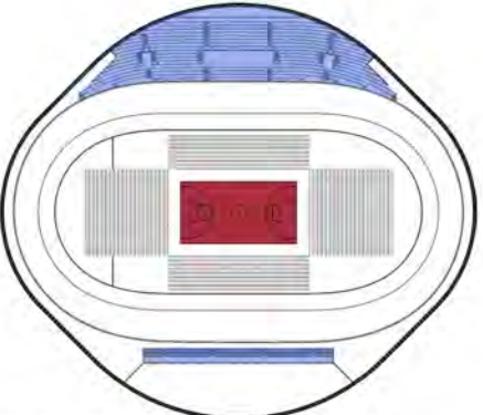
Central Stage / Longitudinal Sport Event 1500 permanent spectators c.200 balcony seats to hospitality and either 800 retractable seats OR 2500 temporary spectator stands to infield
